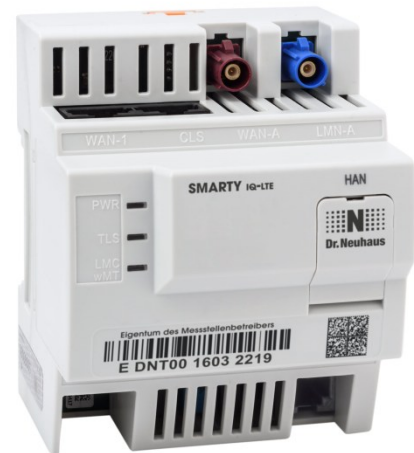
Figure 3: SMARTY IQ-LTE casing and external interfaces
